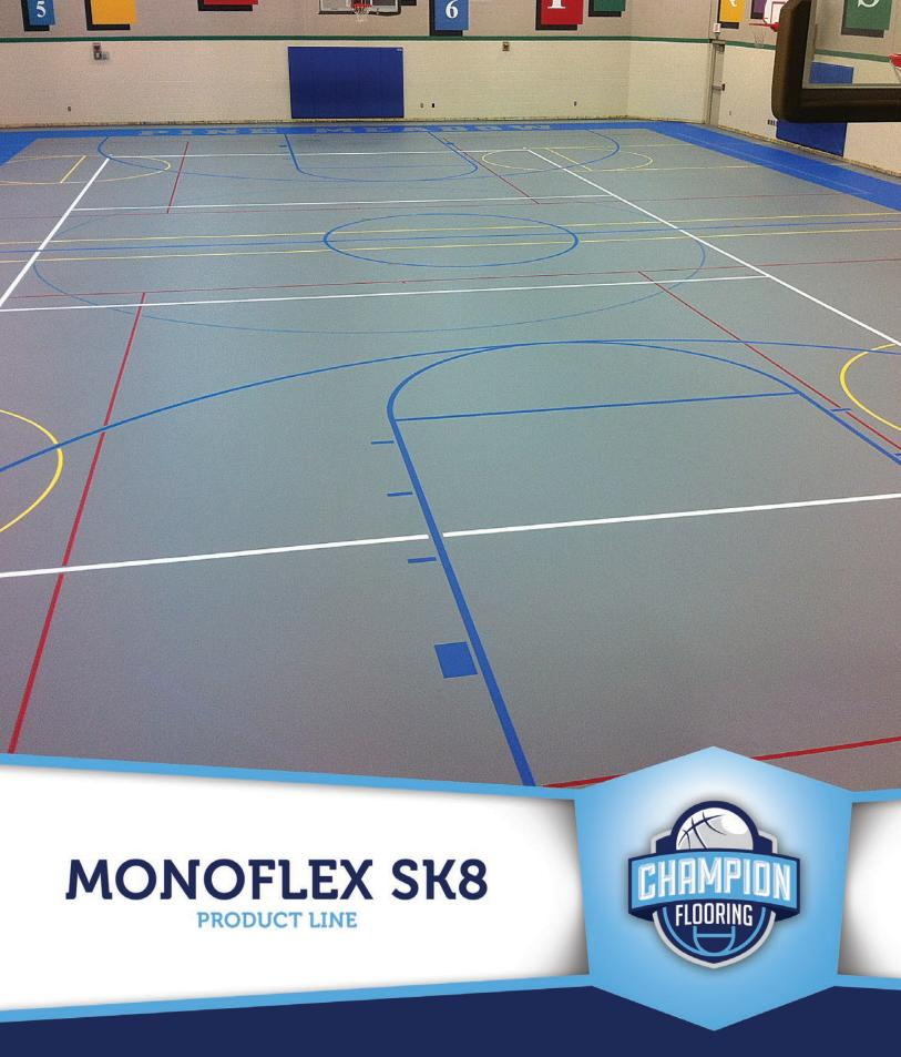
Monoflex SK8 is designed to withstand the high point loads of roller blades and scooters but still meets the needs for a wide variety of other indoor sports. A higher density rubberpad is paired with 3mm of a 60 Shore D urethane to minimize rolling resistance. The Monoflex system incorporates a 92% post-consumer recycled rubber base mat with renewable resource base formula adhesive, scratch coat and wear layer protected by water based topcoat.
